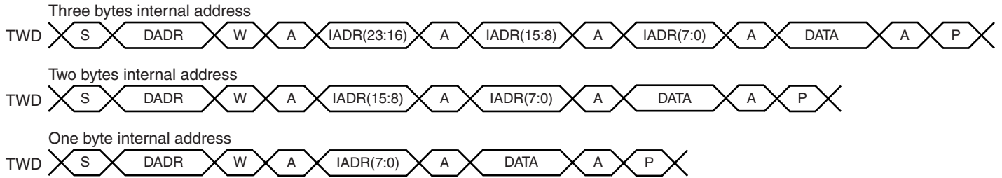
Figure 33-11. Master Write with One, Two or Three Bytes Internal Address and One Data Byte
